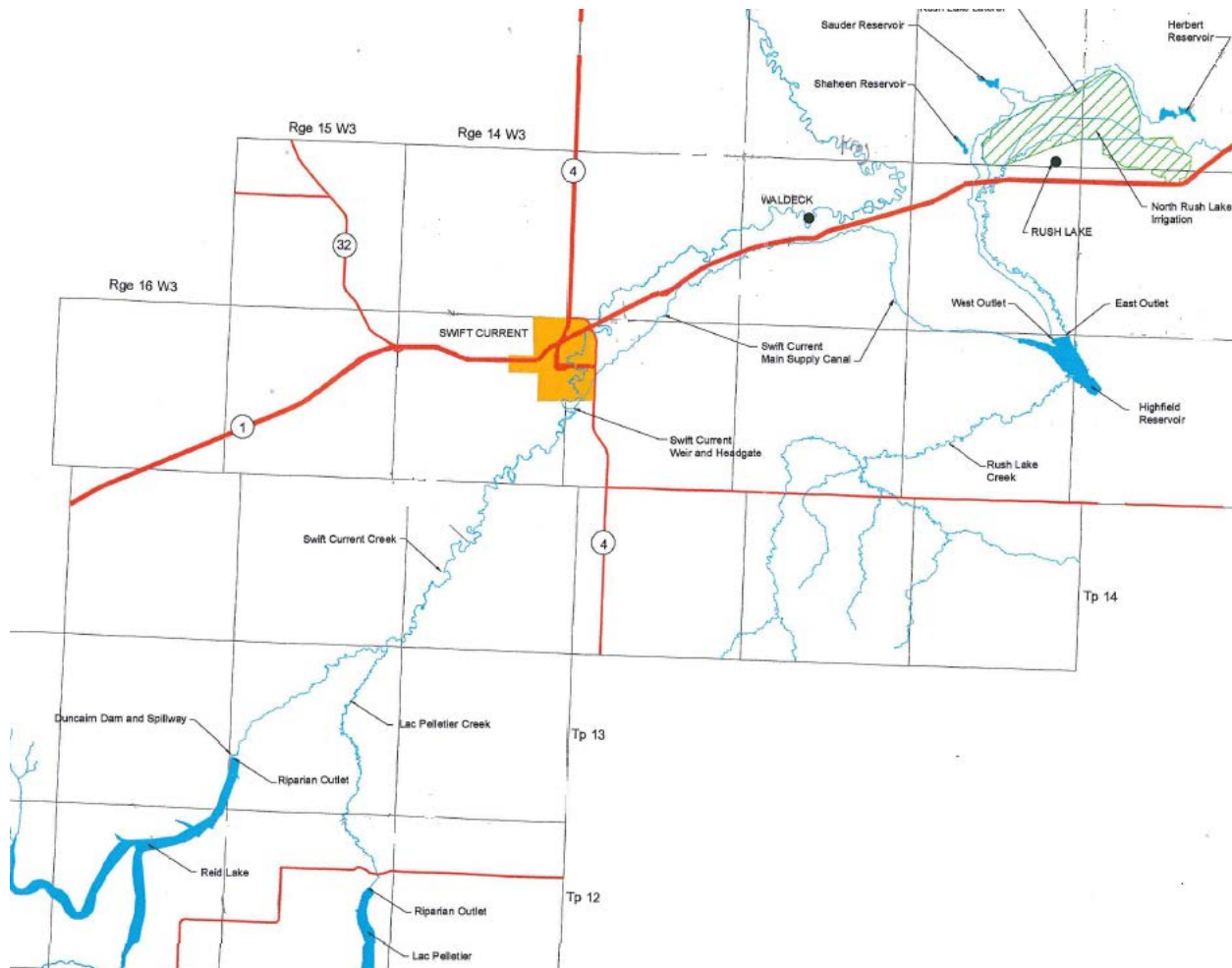
Figure 4.2 Swift Current Diversion Layout (source: Clifton Associates)
