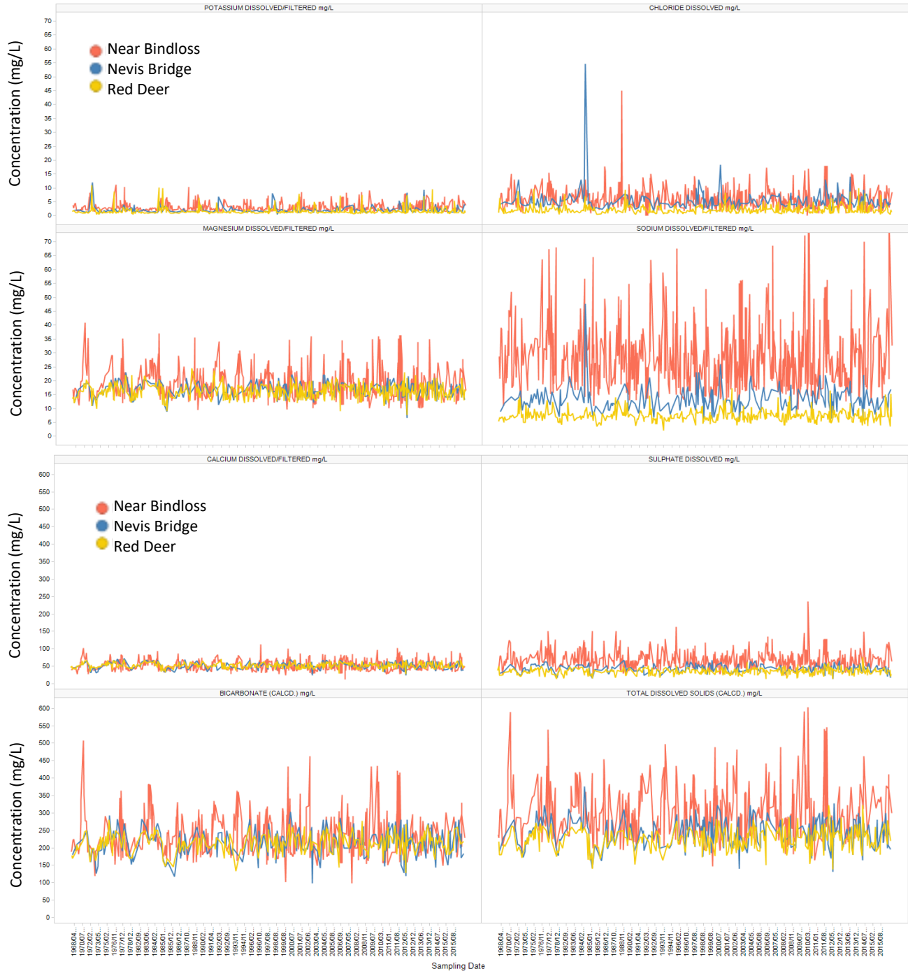
Figure 4. Time series of major ions at three mainstem sites of the Red Deer River
